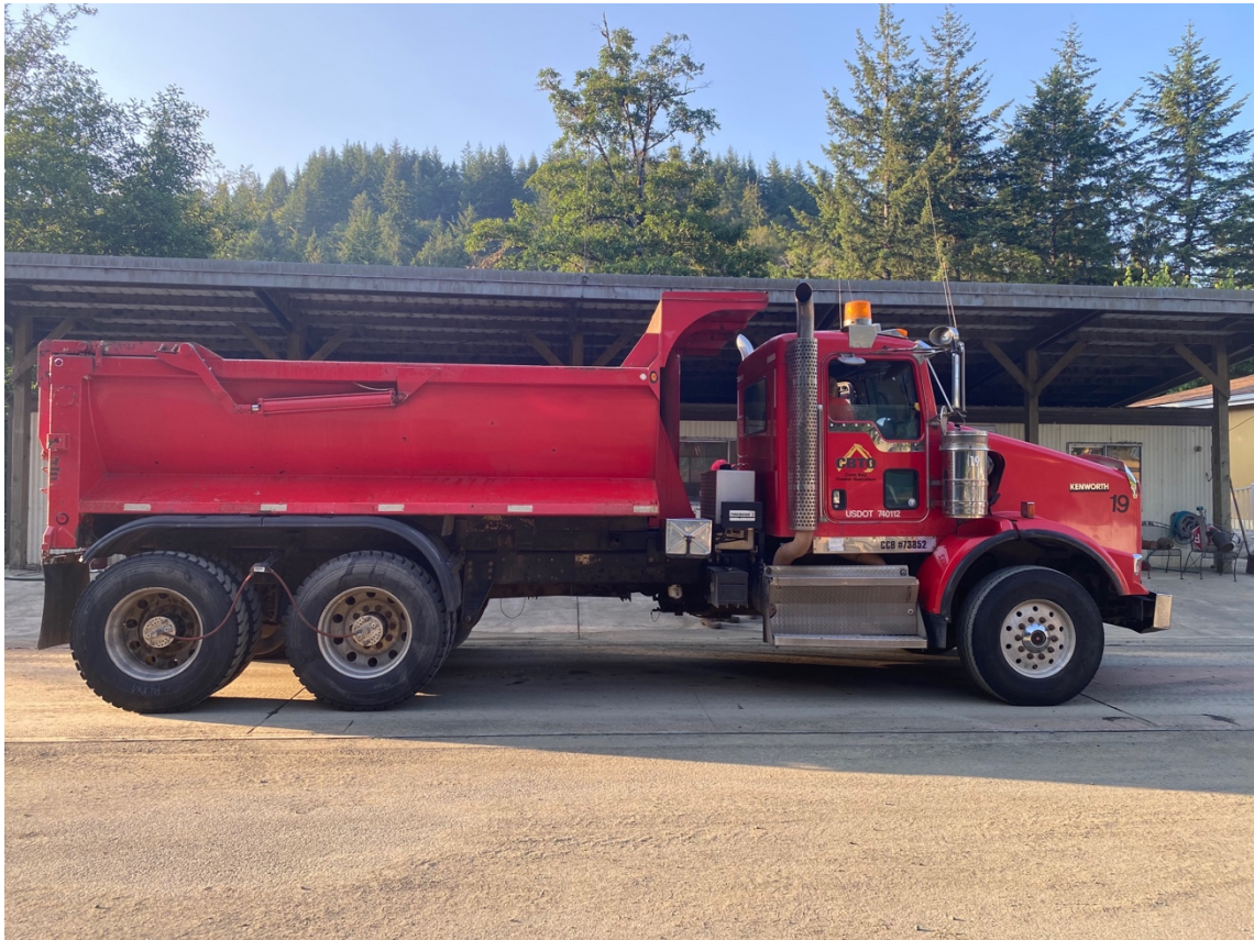
Coos Bay Timber Operators' Kenworth high lift tailgate dump truck and driver, Chris Williams, checking in with Main Rock office, North Bend, Oregon.
