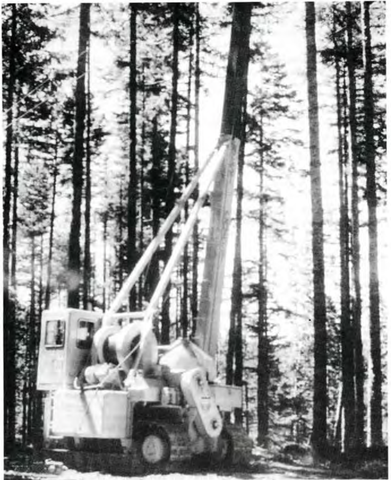
Typical "thinning" yarder, 1966, Howell Ridge Sale. —Elkside Lumber Company photo.
