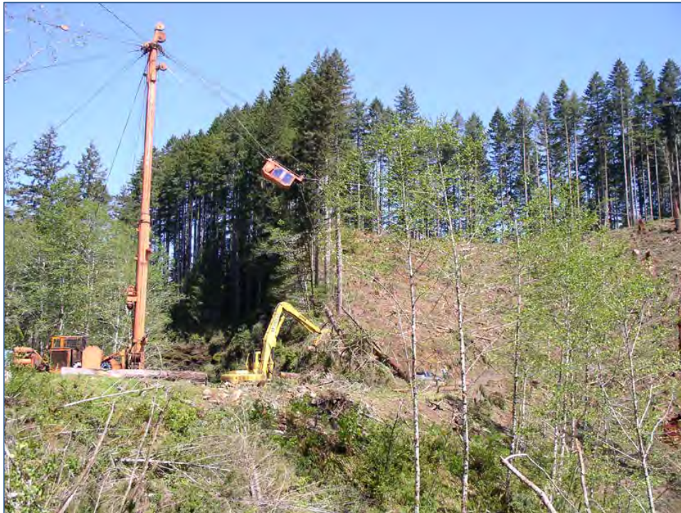
Yarder Operating at Elliott State Forest
