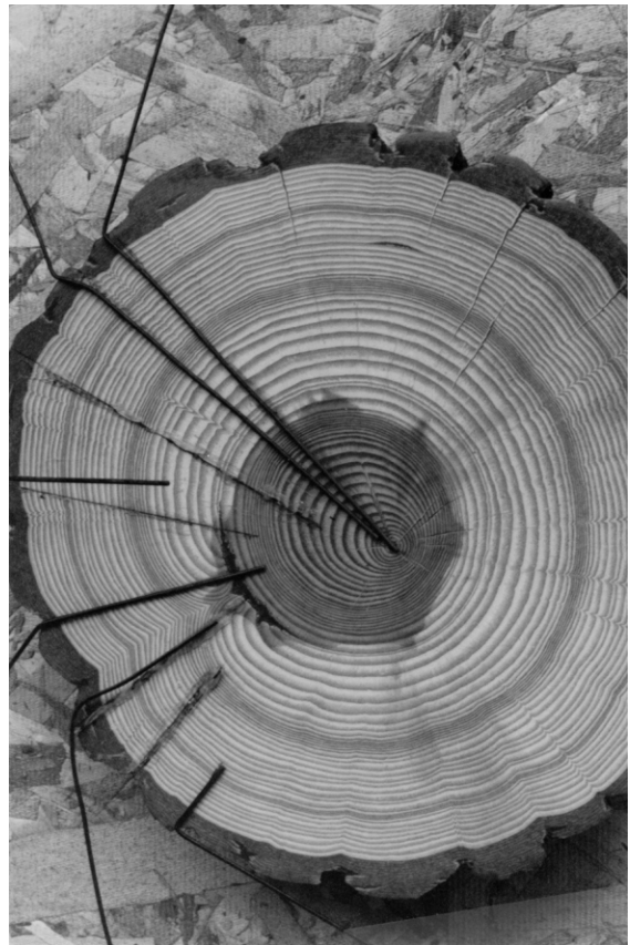
Fig. 8. Section of tree exposing dark mass in tissue (lower left edge of grayish heartwood at center).
