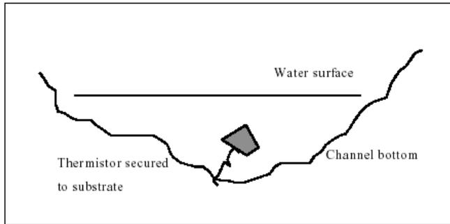
**Figure 6.1. Thermistor placement.**
