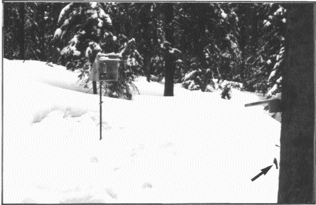
Figure 19—Mechanically triggered camera system used by Bull and others (1992) to monitor presence of marten ( Martes americana Turton). Bait (arrow, lower right) was suspended on the tree to the right under a cover as one modification for winter operation. Camera was a 110 size with flashcube.
