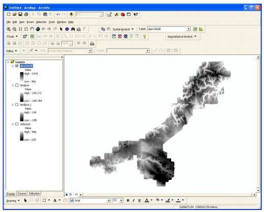
**Figure B-3**–Example showing ten-meter digital elevation model.
