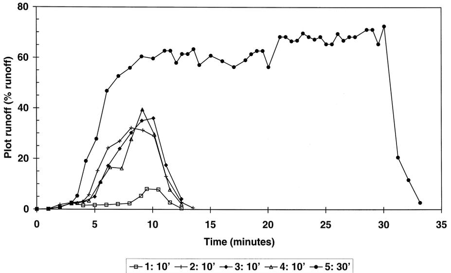
Fig. 3. Results of a rainfall simulation experiment on a sloping *S. tenacissima* covered area ( $2.5 \times 5$  m). Five small events of  $40 \text{ mm h}^{-1}$  are indicated, lasting 10 min except for the last one, which lasted 30 min. The events were divided over two days.
