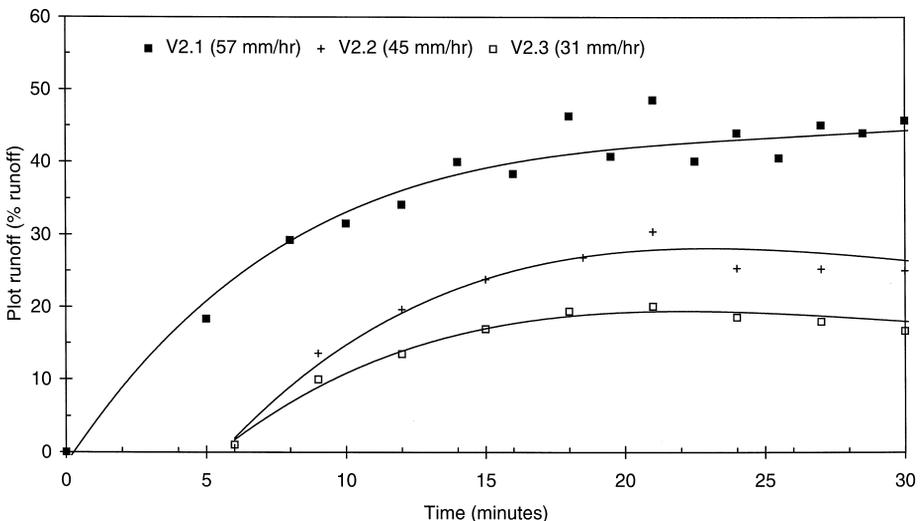
Fig. 6. Runoff curves from rainfall simulation experiments with different rainfall intensities under summer conditions on burnt land at Vilobí, (NE Spain).
