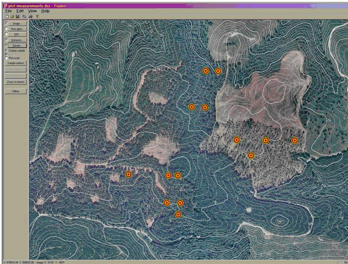
Figure 2. Screenshot of FUSION showing an orthophotograph of the Capitol Forest study site, 20-foot (6.1m) contours created from the digital terrain model, and the location of field plots used in this study.
